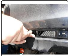
4. Remove (3) nuts from behind each tail light and unplug electrical clip. **Note:** These nuts and plugs are accessed through the trunk. Carefully remove tail lights.
