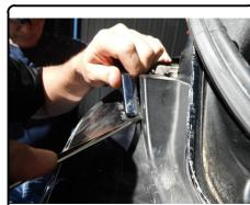
6. Remove (1) fastener from underneath each piece of trim removed in STEP 5.
