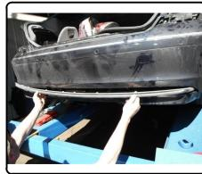
3. Remove (4) fasteners which are located under trim removed in STEP 2.
