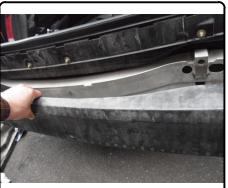
8. Remove bumper beam by removing (6) M10 nuts.
