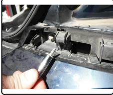
7. Carefully remove bumper cover. Pop sides off first, pull straight back and unplug from vehicle. Remove foam insert and return to vehicle owner.
