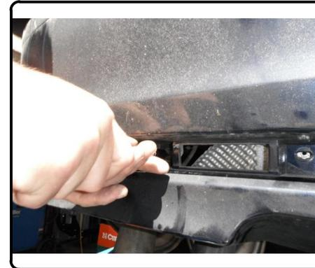
4. Remove (3) nuts from behind each tail light and unplug electrical clip. **Note:** These nuts and plugs are accessed through the trunk. Carefully remove tail lights.
