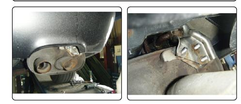
4) Remove plastic rivets from supports on bottom edge of bumper fascia. Rivets are released by first pulling out center post approximately 1/4". Rivet can then be pushed out by hand.
