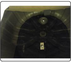
11) Adjust large spacers, trunk strap and hitch to be square with vehicle. Torque all 7/16" fasteners to 70 lb-ft, all 1/2" fasteners to 110 1b-ft.
