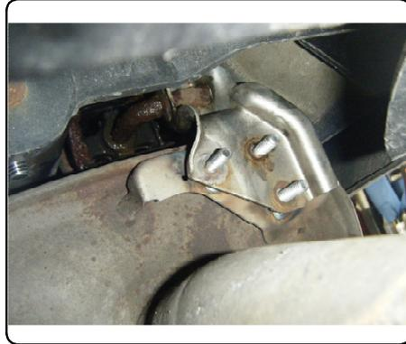
4) Remove plastic rivets from supports on bottom edge of bumper fascia. Rivets are released by first pulling out center post approximately 1/4". Rivet can then be pushed out by hand.
