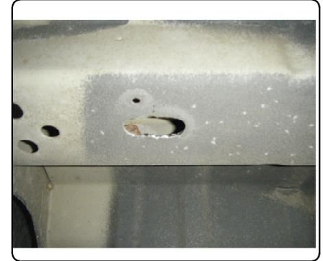
6) Fishwire 7/16" carriage bolt and small spacer block through enlarged access hole in frame rail and out existing hole in frame rail.
