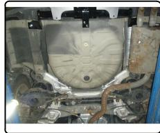
9) Attach trunk strap to top surface of mounting tab on hitch receiver using 1/2" carriage bolts and flange nuts.
