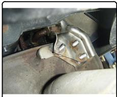
4) Remove plastic rivets from supports on bottom edge of bumper fascia. Rivets are released by first pulling out center post approximately 1/4". Rivet can then be pushed out by hand.
