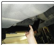
8) Being careful not to push bolts back into frame, lift hitch into position. Install flange nuts, finger tighten.
