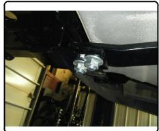
10) Using silicone compound to ensure an air tight seal, install large spacer blocks and 1/2" carriage bolts through drain holes in trunk pan and through holes in trunk strap. Install flange nuts, finger tighten.
