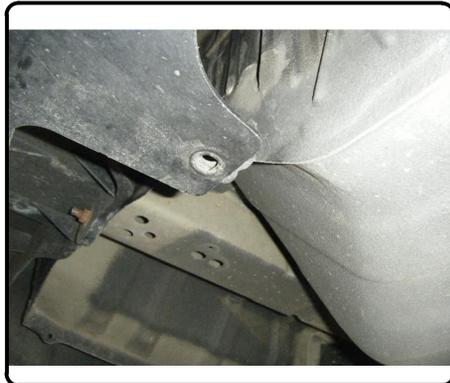
5) Remove material between adjacent holes in frame rail using metal shears or die grinder. Enlarge opening to allow the head of a 7/16" carriage bolt to pass through. Repeat for other side of vehicle.
