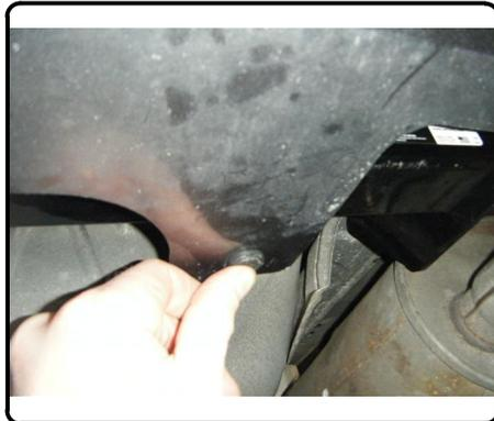
13) Raise exhaust and re-attach muffler hanger bracket/brackets.
