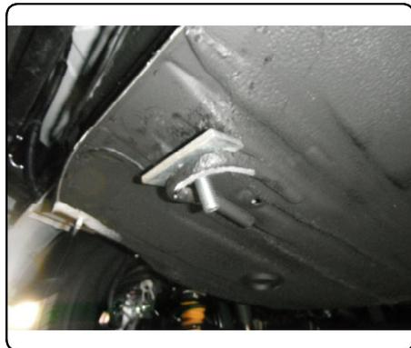
6. Raise hitch into position and secure hitch to tow loop with 1/2" flange nut. Remove fishwires and attach 7/16" hex flange nuts.
