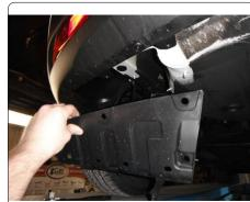
2. Lower exhaust by removing two rubber exhaust hangers. (See RUBBER ISOLATOR REMOVAL DIAGRAM on page 2)
