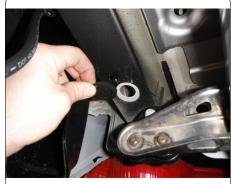
4. Reverse fishwire a 7/16" carriage bolt with a CM-SP2 spacer into each hole which a plug was removed from in step 3. (See REVERSE PULL FISHWIRE TECHNIQUE on page 2) **Note:** Leave fishwires attached to prevent loss of hardware inside frame.
