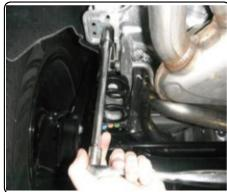
2. Reverse fishwire 1/2"-13 x 1 1/2" carriage bolts and CM-SP17 spacers into driver and passenger side frame rails.
