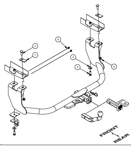
1. Remove existing bolt from driver side exhaust hanger. Return bolt to vehicle owner.
