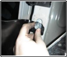
4. Torque 1/2"-13 hardware to 110 lb-ft and M12-1.50 hardware to 83 lb-ft.
