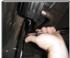
4. Reverse fishwire 1/2" x 1 1/2" carriage bolts and CM-SP17 spacers into holes enlarged in Step 3. Install 1/2" x 1 3/4" carriage bolt and CM-SP4 spacer through top of vehicle tow loop.
