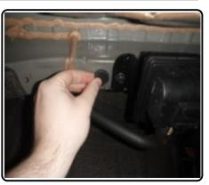
2. Trim heat shield to allow access to round hole on passenger side of vehicle.
