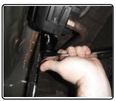
6. Raise exhaust back into position and reattach the rubber isolators. Install is complete.
