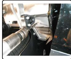
3. Fishwire 7/16" carriage bolt with CM-SP2 spacer through the access hole in the passenger side frame rail into the hole enlarged in step 2. See FISHWIRE TECHNIQUE on page 2. **Note:** Leave fishwires attached to all 7/16" hardware to prevent loss of hardware inside frame rail.
