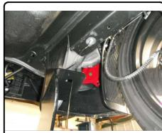
6. Place 1/2" carriage bolt with CM-SP6 spacer through tow loop and hitch and secure hitch to tow loop with 1/2" flange nut.
