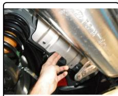
2. Remove one rubber plug from each frame rail and return to vehicle owner. Enlarge rearmost hole on passenger side frame rail using a 1/2" drill bit.
