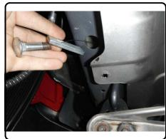
4. Reverse fishwire 7/16" carriage bolt with CM-SP2 spacer into access hole on both sides. See REVERSE PULL FISHWIRE TECHNIQUE on page 2.
