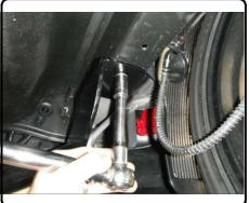
8. Reinstall the two M8 nuts removed in step 1.
