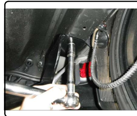
8. Reinstall the two M8 nuts removed in step 1.
