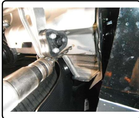
3. Fishwire 7/16" carriage bolt with CM-SP2 spacer through the access hole in the passenger side frame rail into the hole enlarged in step 2. See FISHWIRE TECHNIQUE on page 2. **Note:** Leave fishwires attached to all 7/16" hardware to prevent loss of hardware inside frame rail.
