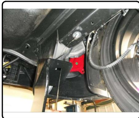
6. Place 1/2" carriage bolt with CM-SP6 spacer through tow loop and hitch and secure hitch to tow loop with 1/2" flange nut.
