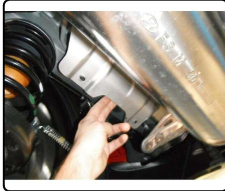
2. Remove one rubber plug from each frame rail and return to vehicle owner. Enlarge rearmost hole on passenger side frame rail using a 1/2" drill bit.
