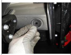
Raise hitch into position with the tow loop mounting tab resting on top of the tow hook. Mark the forward hole on the driver side frame rail and drill with a 15/32" drill bit. Remove hitch. <u>Note</u>: Hyundai Accent sedan does not require drilling.
