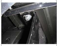
5. Install the remaining 3/8" hardware with (1) CM-SP34 spacer onto the vehicle tow loop, as shown above.
