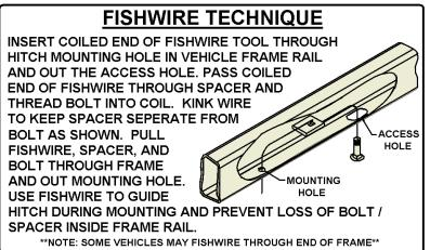
**REVERSE PULL FISHWIRE TECHNIQUE** ATTACH FISHWIRE TO CARRIAGE BOLT AND SLIDE SPACER ONTO FISHWIRE. PUSH THE BOLT THRU THE HOLE FOLLOWED BY THE SPACER (AS SHOWN). PULL BOLT BACK INTO POSITION, PROTRUDING FROM THE FRAME.
