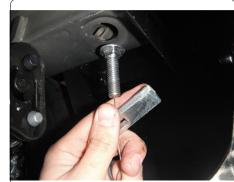
Raise the hitch back into position. Be careful not to push the carriage bolts back into the frame. Loosely install (3) 7/16" hex flange nuts.
