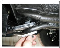
6. Torque all 3/8" fasteners to 45 lb-ft and all 7/16" fasteners to 70 lb-ft.
