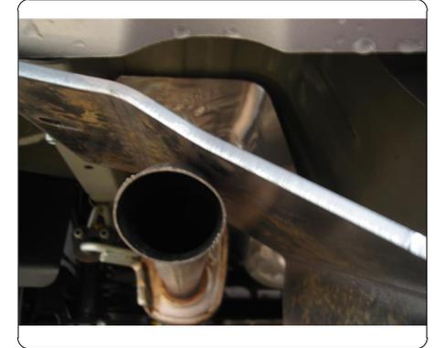
2. Raise hitch into position, lifting driver side first over tailpipe, then lifting passenger side.
