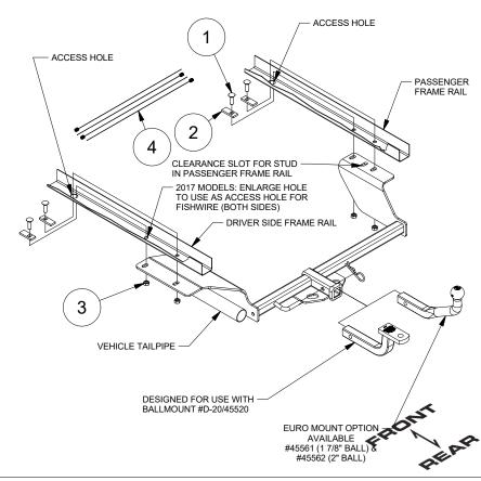
1. Fishwire CM-SP2 spacers and 7/16-14 carriage bolts through access hole in frame rail and down through attachment hole, (2) places, each side.
