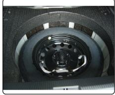
5. Remove the middle plug on the driver side of the spare tire well. Return plug to vehicle owner.
