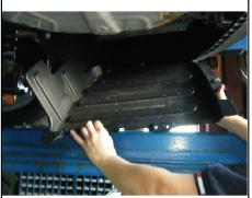
2. Lower the exhaust by removing the (2) hex flange bolts from exhaust hanger bracket. Return to vehicle owner. (Leave the muffler attached to the exhaust hanger bracket.)
