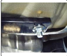
9. Torque all M8 hardware to 17 ft-lbs., all 7/16" hardware to 70 ft-lbs. and all 1/2" hardware to 110 ft-lbs. Trim rear underbody panel to clear the passenger side plate as shown in the Underbody Panel Trim Diagram. Reinstall the underbody panel using the torx head screws and hex nuts removed in Step 1.
