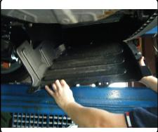
Lower the exhaust by removing the (2) hex flange bolts from exhaust hanger bracket. Return to vehicle owner. (Leave the muffler attached to the exhaust hanger bracket.)
