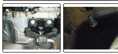
8. Use silicone caulk (or equivalent) to seal the tire well plug hole from exhaust fumes and water by putting a bead around the CM-SP62 spacer. Place the CM-SP62 spacer onto the hole and put a bead of caulk around the square hole. Install a 1/2" carriage bolt and secure with a hex flange nut from under the vehicle as shown.
