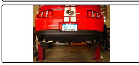
4. Raise hitch into position, feeding ends of fishwires through mounting holes on hitch frame brackets. Using attached fishwires, pull bolts through holes in side of frame rails and hitch frame brackets. Secure with 7/16" flange nuts, as shown.
