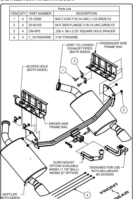
1. Remove the rearmost rubber isolator on both mufflers. (See RUBBER ISOLATOR REMOVAL DIAGRAM).
