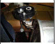
2. Lower exhaust by loosening the strap which fastens the exhaust pipes together behind the muffler and gently pulling mufflers downward to allow access to frame rails.
