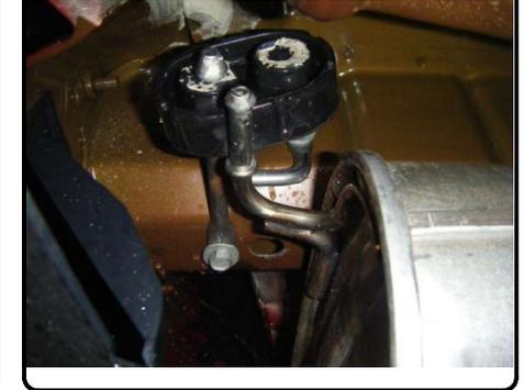
2. Lower exhaust by loosening the strap which fastens the exhaust pipes together behind the muffler and gently pulling mufflers downward to allow access to frame rails.
