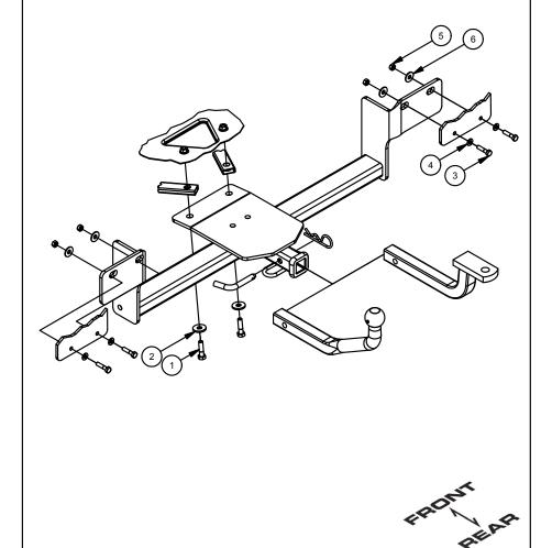
1. Remove (1) fascia screw per side of vehicle. Middle screw will remain attached. Retain screws for reinstallation.
