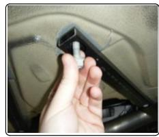
5. Install supplied M8 hex bolts and flat washers through threaded holes in bumper brackets where factory M8 hardware was removed in Step 3.
