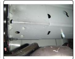
4. Raise driver side plate into position on driver side frame rail and loosely fasten with 1/2" flange nut.
