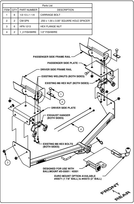
1. Remove (2) exhaust hangers by unbolting (4) M8 hex bolts and (2) M8 hex nuts.
