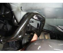
2. Lower exhaust by removing (2) forward rubber isolators.
