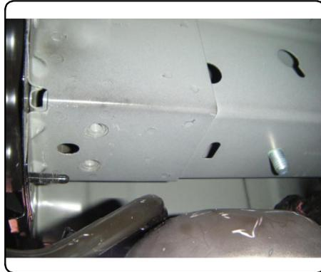
4. Raise driver side plate into position on driver side frame rail and loosely fasten with 1/2" flange nut.
