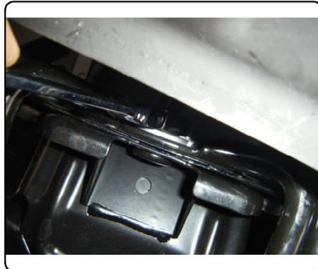
9. Raise hitch into position and fasten to side plates with 1/2" hardware, as shown above. Torque all 1/2" hardware to 75 ft-lbs. Reinstall (2) rubber isolators which were removed in STEP 1.
