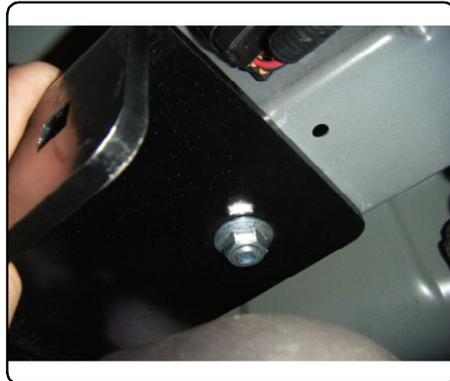
5. Place exhaust hanger back into position. (Plate will now be sandwiched between frame rail and exhaust hanger.) Reinstall (1) M8 hex nut which was removed in STEP 1.
