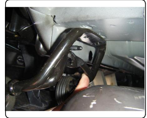
2. Lower exhaust by removing (2) forward rubber isolators.
