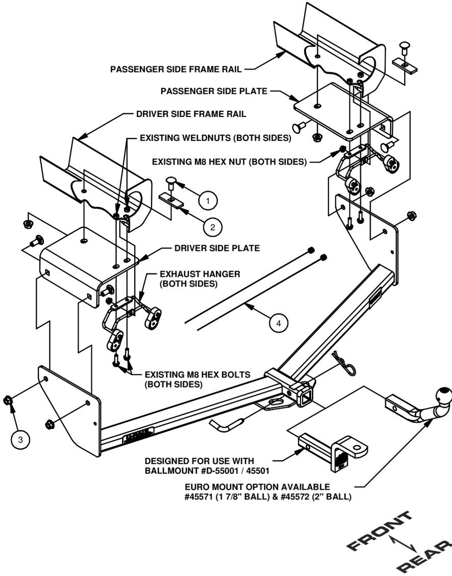
1. Remove (2) exhaust hangers by unbolting (4) M8 hex bolts and (2) M8 hex nuts.
