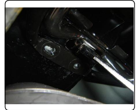
6. Reinstall (2) M8 hex bolts which were removed in STEP 1. Repeat STEPS 4-6 with passenger side plate.
