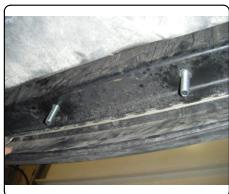
Raise hitch back into position and secure with 1/2"-13 flange nuts. Torque all 1/2" fasteners to 75 ft-lbs.
