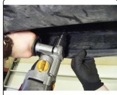
5. Fishwire 1/2"-13 x 2" carriage bolts and SP6 spacers through the access holes between the fascia and the back of the bumper beam and into holes drilled in STEP 4. (See FISHWIRE TECHNIQUE DIAGRAM on page 2)
