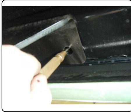
4. Lower hitch and drill hole locations with 17/32" drill bit.
