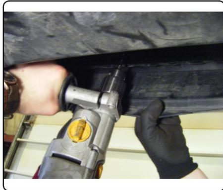
5. Fishwire 1/2"-13 x 2" carriage bolts and SP6 spacers through the access holes between the fascia and the back of the bumper beam and into holes drilled in STEP 4. (See FISHWIRE TECHNIQUE DIAGRAM on page 2)
