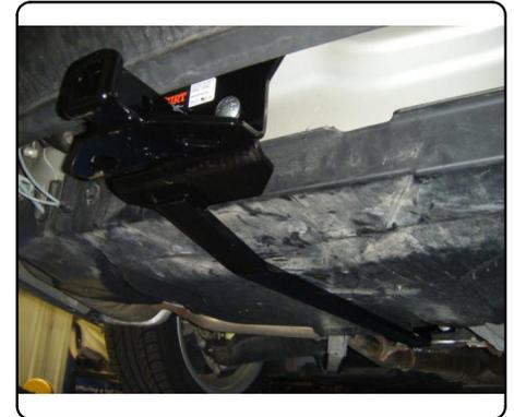
**11189****MERCEDES BENZ E-350 WAGON****6/17/2014****GROSS LOAD CAPACITY WHEN USED AS A WEIGHT CARRYING HITCH: 2,000 LBS. TRAILER WEIGHT & 200 LBS. TONGUE WEIGHT.**
