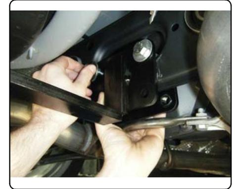
2. Raise hitch past fascia lip and secure to mounting strap using 1/2"-13 x 1 1/4" carriage bolts and 1/2"-13 flange nuts.
