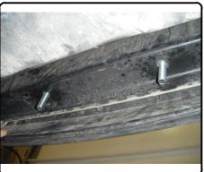
6. Raise hitch back into position and secure with 1/2"-13 flange nuts. Torque all 1/2" fasteners to 75 ft-lbs.
