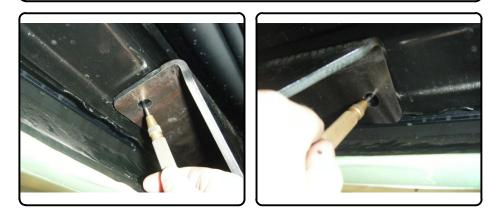
4. Lower hitch and drill hole locations with 17/32" drill bit.
