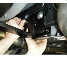
2. Raise hitch past fascia lip and secure to mounting strap using 1/2"-13 x 1 1/4" carriage bolts and 1/2"-13 flange nuts.
