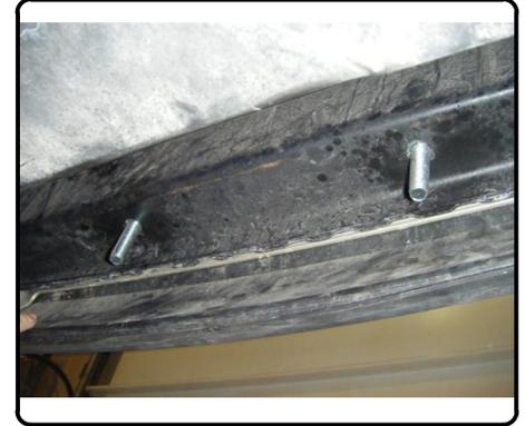
6. Raise hitch back into position and secure with 1/2"-13 flange nuts. Torque all 1/2" fasteners to 75 ft-lbs.
