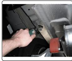
FISHWIRE TECHNIQU INSERT COILED END OF FISHWIRE TOOL THROUGH HITCH MOUNTING HOLE IN VEHICLE FRAME RAII AND OUT THE ACCESS HOLE. PASS COILED END OF FISHWIRE THROUGH SPACER AND THREAD BOLT INTO COIL. KINK WIRE TO KEEP SPACER SEPERATE FROM BOLT AS SHOWN. PULL FISHWIRE, SPACER, AND BOLT THROUGH FRAME AND OUT MOUNTING HOLE USE FISHWIRE TO GUIDE HOLE HITCH DURING MOUNTING AND PREVENT LOSS OF BOLT / SPACER INSIDE FRAME RAIL. "NOTE: SOME VEHICLES MAY FISHWIRE THROUGH END OF FRAME
