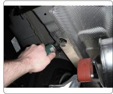
FISHWIRE TECHNIQUE INSERT COILED END OF FISHWIRE TOOL THROUGH HITCH MOUNTING HOLE IN VEHICLE FRAME RAIL AND OUT THE ACCESS HOLE. PASS COILED END OF FISHWIRE THROUGH SPACER AND THREAD BOLT INTO COIL. KINK WIRE TO KEEP SPACER SEPERATE FROM BOLT AS SHOWN. PULL FISHWIRE, SPACER, AND BOLT THROUGH FRAME AND OUT MOUNTING HOLE. USE FISHWIRE TO GUIDE HOLE HITCH DURING MOUNTING AND PREVENT LOSS OF BOLT / SPACER INSIDE FRAME RAIL. \*\*NOTE: SOME VEHICLES MAY FISHWIRE THROUGH END OF FRAME\*
