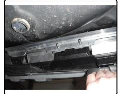
4. Raise hitch into position and loosely secure the rear of the hitch to the fasteners installed in Step (3) with a 7/16-14 flange nut and a 3/8-16 flange nut. Secure the front of the hitch to the existing weldnuts with M10-1.5 x 25mm hex bolts and 7/16" conical toothed washers.
