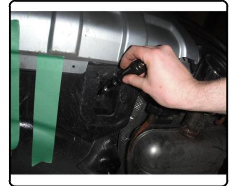
2. Mark and trim the under body panel. **Note:** Dimensions are approximate, confirm fit prior to trimming.
