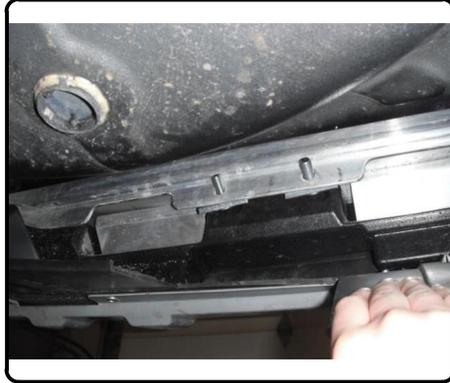
4. Raise hitch into position and loosely secure the rear of the hitch to the fasteners installed in Step (3) with a 7/16-14 flange nut and a 3/8-16 flange nut. Secure the front of the hitch to the existing weldnuts with M10-1.5 x 25mm hex bolts and 7/16" conical toothed washers.
