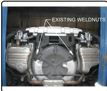
5. Torque all 3/8" fasteners to 45 ft-lbs. Torque all 7/16" fasteners to 59 ft-lbs. Torque all M10 fasteners to 45 ft-lbs. Reinstall the (2) fascia nuts removed in Step (1).
