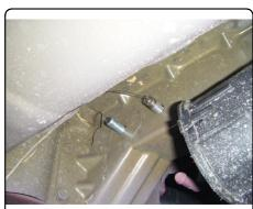
4. Thread fishwires through appropriate mounting holes and raise hitch into position.
