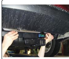
5. Secure hitch to vehicle with (4) 1/2" flange nuts.
