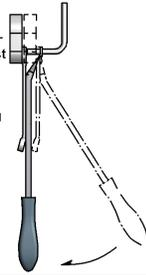
Note: Using a spray lubricant or soapy water on the hanger rod and the rubber isolator helps removal.
