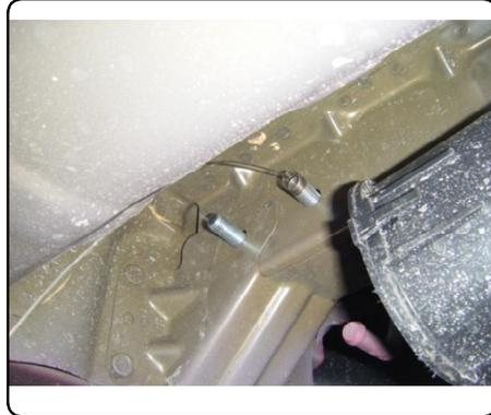
4. Thread fishwires through appropriate mounting holes and raise hitch into position.
