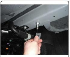
6. Mark heat shield for trimming and confirm the fit. Trim heat shield and reattach using (4) fasteners removed in Step (2).
