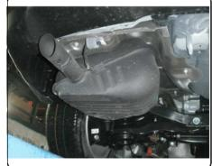
2. Remove the heat shield by removing (6) fasteners.
