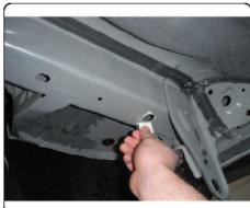
4. Fishwire 7/16-14 carriage bolts and SP7 spacers through the access holes and out the rear-most holes in the frame rails, both sides.
