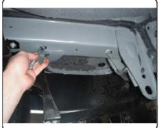
5. Reverse fishwire 7/16-14 carriage bolts and SP7 spacers in the access holes, both sides.
