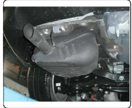
2. Remove the heat shield by removing (6) fasteners.
