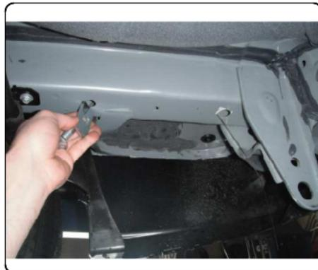
5. Reverse fishwire 7/16-14 carriage bolts and SP7 spacers in the access holes, both sides.
