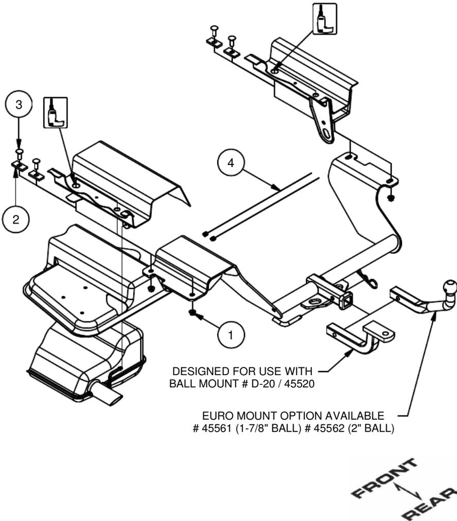
1. Lower exhaust by removing (3) rubber exhaust hangers.
