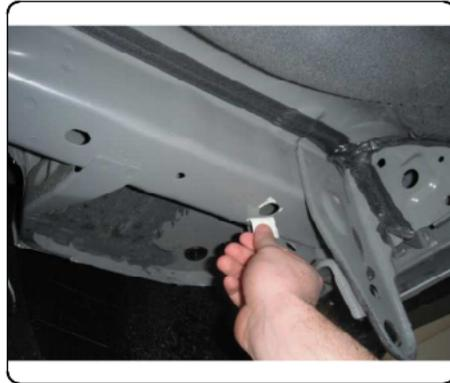
4. Fishwire 7/16-14 carriage bolts and SP7 spacers through the access holes and out the rear-most holes in the frame rails, both sides.
