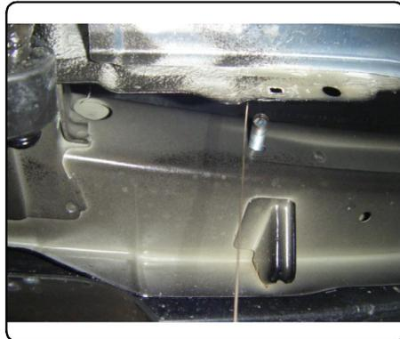
7. Thread fishwires through appropriate mounting holes on hitch and raise hitch into position.
