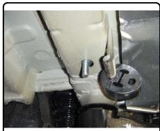
6. Fishwire (2) 7/16" carriage bolts and (2) CM-SP2 spacers into position in bumper beam through access holes. See FISHWIRE TECHNIQUE on page 2. (**Note:** Leave fishwires attached to hardware to prevent loss in beam.)
