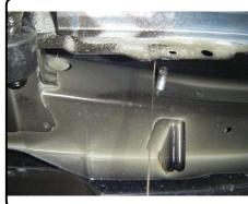
7. Thread fishwires through appropriate mounting holes on hitch and raise hitch into position.
