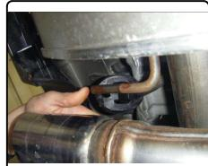
2. Remove (2) brackets which hold fascia to vehicle. These will be reinstalled in step 8.
