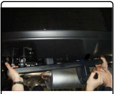
4. Remove forward most rubber plug from each frame rail.
