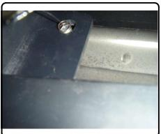
8. Torque all 7/16" hardware to 70 ft-lbs. Reinstall (2) brackets which were removed in step 2.
