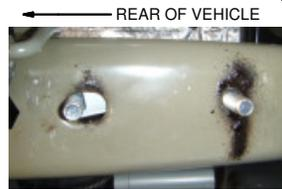
BOLTS INSTALLED IN FRAME RAIL
