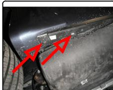
4. Pull back wheel well liner to remove (1) hex head fastener.
