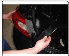
10. Carefully pull off tail lights by pulling straight back.
