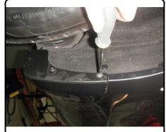
3. Remove (2) push fasteners from wheel well liner and (2) fasteners from bottom of bumper cover.
