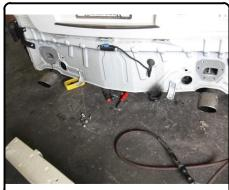
14. Raise hitch and bumper beam into position and secure to vehicle with the included (12) 3/8" conical tooth washers and (12) M8 hex bolts.
