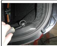
8. Pull back inner trunk liner to expose and remove (2) hex nuts. It may ease the process to remove push fasteners from inner liner. Repeat on other side.
