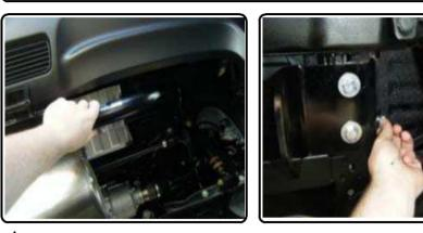
4. Torque M12-1.25 hardware to 86 lb-ft and M10-1.25 hardware to 48 lb-ft.
