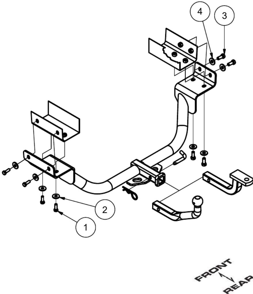
1. Remove existing tow loop from passenger side of vehicle. Return tow loop and hardware to vehicle owner.
