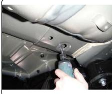
5. Fishwire 7/16-14 x 1 1/2" carriage bolts and CM-SP11 spacers through access holes and out mounting holes in both frame rails.
