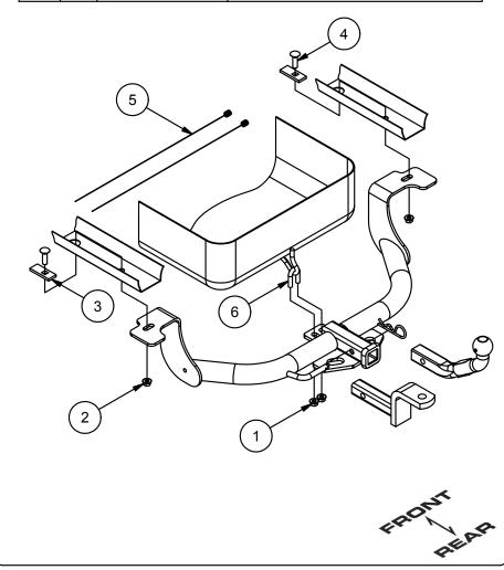
1. Lower exhaust by removing (2) rubber isolators for single exhaust vehicles and (4) isolators for dual exhaust vehicles.
