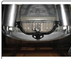
8. Trim heat shield(s) around hitch. Reinstall heat shield(s) with hardware removed in Step (2). **Note:** Dimensions are approximate, confirm fit prior to trimming.
