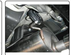
2. Remove heat shield(s) by removing (4) screws per shield. Save screws and shield(s) for reinstallation later.
