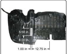
4. Check if hardware can be inserted through access holes in frame rails. If not, enlarge the holes with a die grinder or rotary tool until hardware can pass through.
