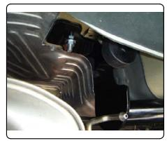
9. Raise exhaust and reattach rubber isolators. If under body panel is present, resecure using fasteners removed in Step (3).
