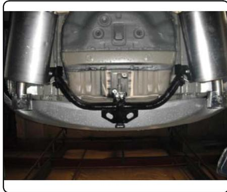
8. Trim heat shield(s) around hitch. Reinstall heat shield(s) with hardware removed in Step (2). **Note:** Dimensions are approximate, confirm fit prior to trimming.
