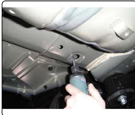
5. Fishwire 7/16-14 x 1 1/2" carriage bolts and CM-SP11 spacers through access holes and out mounting holes in both frame rails.
