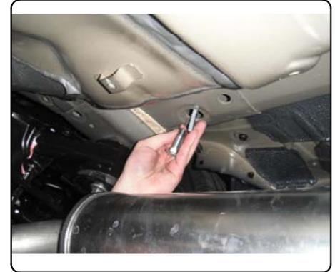
6. Insert 3/8" U-bolt through tow loop. Raise hitch into position and secure it with 7/16-14 hex flange nuts on the carriage bolts and 3/8-16 hex flange nuts on the U-bolt. If underbody panel is present you will need to raise it with the hitch.
