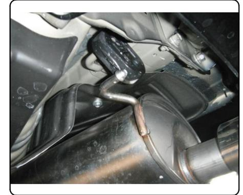
2. Remove heat shield(s) by removing (4) screws per shield. Save screws and shield(s) for reinstallation later.
