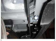
4. Raise passenger side plate over the exhaust and slide it past the exhaust hanger. Raise driver side plate past the vapor canister and secure both plates using 7/16-14 flange nuts. <u>Note</u>: When raising hitch into position you may have to push bolts part way back into the frame to get the plates into position. You may use fishwires to guide hitch druing mounting to prevent the loss of bolts and spacers inside the frame rail.
