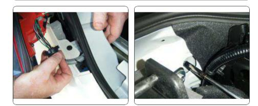
A. Remove the tail lights. Remove the (4) clips holding the bumper. Place the bumper cover where it will not be damaged. Retain all hardware for reinstallation.
