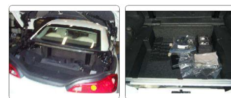
A. Remove the plastic panel at the rear of the trunk by removing (4) clips and (2) screws. Also detach the electrical connection for the interior light.
