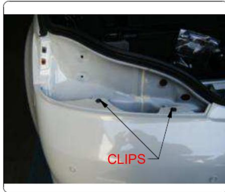
B. To trim the bumper cover, first temporarily remove the license plate. Locate the (2) rectangular holes cut through the cover. Lay out a rectangular area that is 1 1/2" by 6". Center the rectangle on the vehicle and position it 2 1/4" below the rectangular holes. Trim out the area using a rotary tool with a cutoff wheel. Remove (2) clips on the bottom of the bumper cover.
