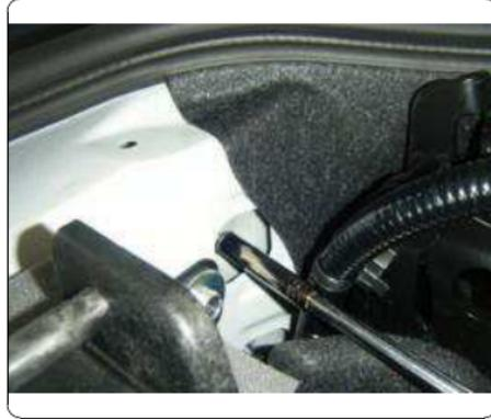
A. Remove the tail lights. Remove the (4) clips holding the bumper. Place the bumper cover where it will not be damaged. Retain all hardware for reinstallation.
