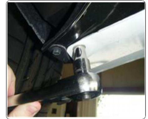
A. Remove (3) clips and (1) screw from the driver and passenger side tire wells.
