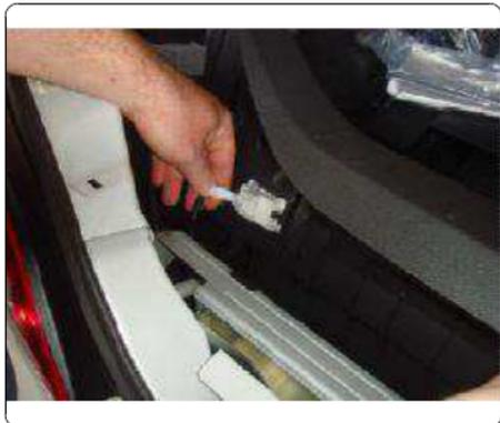
A. Remove the (2) plastic bottom side panels by removing (1) clip per panel.
