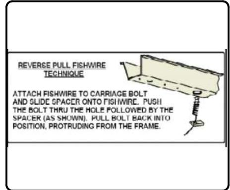
6. Raise hitch over the exhaust and slide it past the exhaust hanger. Secure hitch using 7/16-14 flange nuts. **Note:** When raising hitch into position you may have to push bolts part way back into the frame to get the plates into position. You may use fishwires to guide hitch during mounting to prevent the loss of bolts and spacers inside the frame rails.
