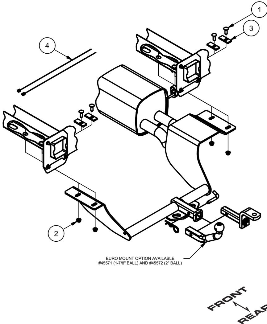
1. Lower exhaust by removing (2) rubber isolators from the hangers attached to the frame.
