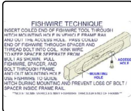
5. Reverse fishwire 7/16-14 x 1 1/4" carriage bolt and SP11 spacer into the rear most hole, both sides.
