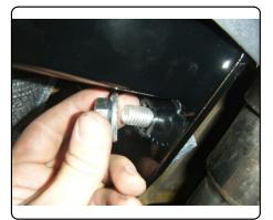
4. Secure exhaust hanger brackets and hitch to frame using the supplied M8 fasteners and 3/8" conical tooth washers.
