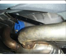
2. Raise hitch into position. (NOTE: Hitch will be sandwiched between frame and exhaust hanger brackets)
