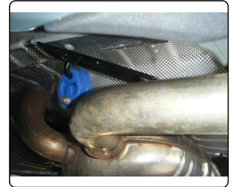
2. Raise hitch into position. (NOTE: Hitch will be sandwiched between frame and exhaust hanger brackets)
