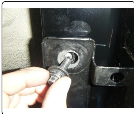
5. Torque all M8 fasteners to 24 ft-lbs and all 1/2" hardware to 110 ft-lbs.
