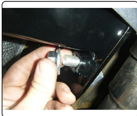
4. Secure exhaust hanger brackets and hitch to frame using the supplied M8 fasteners and 3/8" conical tooth washers.
