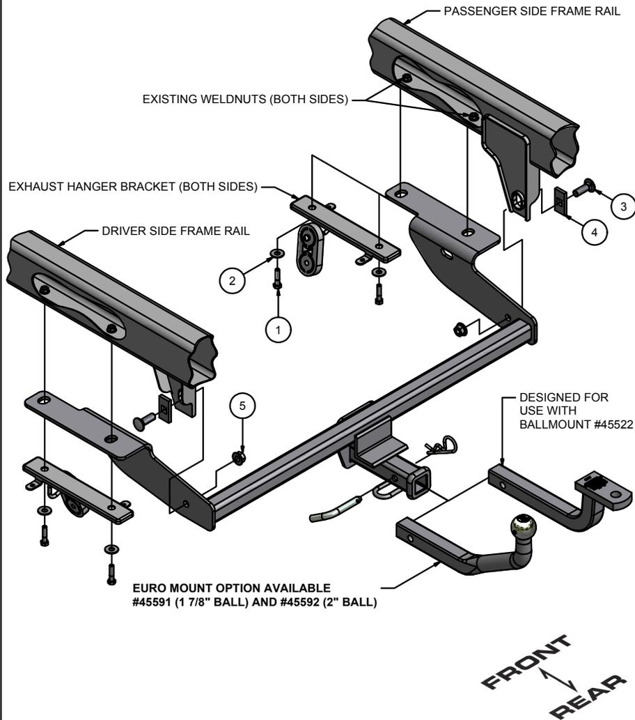
1. Lower exhaust by removing (2) M8 fasteners from each exhaust hanger bracket. Return (4) M8 fasteners to vehicle owner.
